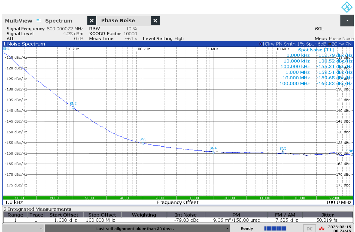
Figure 7: ADC Sampling Clock Characterization (500 MHz), 1 kHz to 100 MHz Integration Bandwidth, Rohde & Schwarz FSWP analyzer
